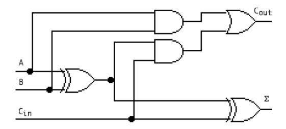
Suppose that the propagation delays for the and and or gates are 0.1 ns each, while that for the xors is 0.2 ns. (XOR requires a more complex circuit). Then the delay from A or B to Cout is  $\max(0.1 + 0.1 \text{ ns}, 0.2 + 0.1 + 0.1 \text{ ns}) = \max(0.2, 0.4 \text{ ns}) = 0.4 \text{ ns}.$
